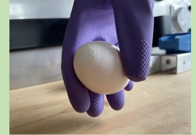
Harvest Moon (6) Dexterous Adaptive Robotic Gripper
