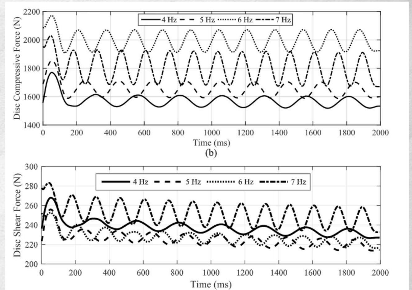
Compressive and Shear Forces in the Spine at Different Vibration Frequencies [1]
