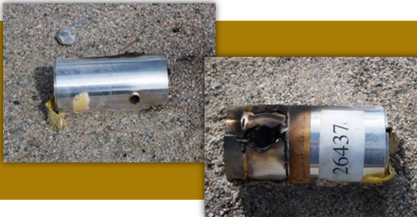
Bullet Impact in generic hardware No damage to end closure or copper liner Mild response to 0.50 cal round
