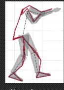
Align human motion model with kinematic model
