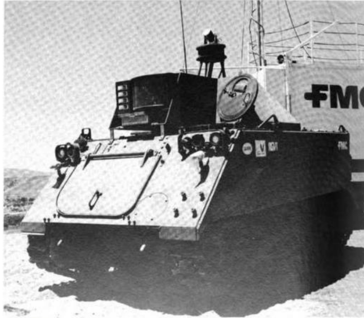
FMC Corporation's AGVT (advanced ground vehicle technology) demonstrator, based on an M113-series armored personnel carrier.
