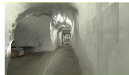
Figure 9. A group of three autonomous robotic systems generated without operator intervention a map of this underground facility. The system autonomously coordinated and merged the resulting map. Both 2D maps and 3D textured maps were generated.
