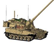
**WHAT**: Upgraded 155mm self-propelled artillery system and munitions to provide increased ranges and survivability. ERCA capability includes cannon, propellant, and ammunition upgrades.
