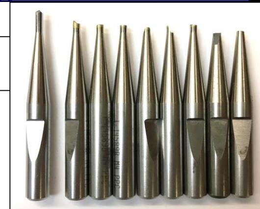
Actual broken punches seen in production
