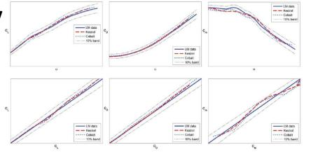
Figure 2. F-16C CFD (*Kestrel* and *Cobalt*, full-scale) with LEF = 0 degrees vs. LM Performance Data with LEF = 0 degrees for C<sub>L</sub>, C<sub>D</sub> and C<sub>m</sub>, Mach 0.9.
