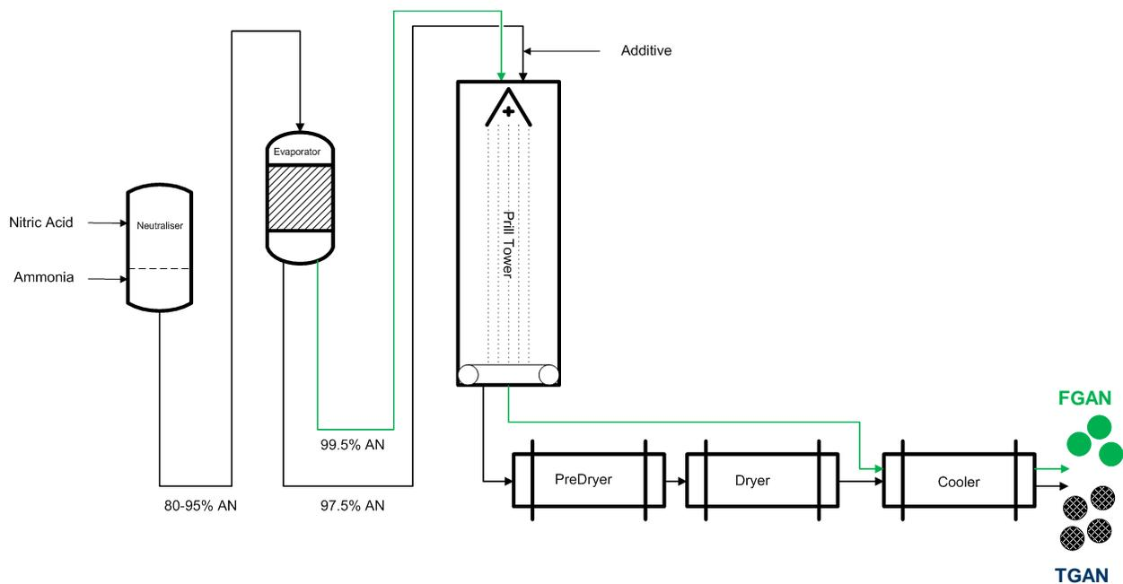
Figure 1. Schematic for the Manufacture of Ammonium Nitrate
