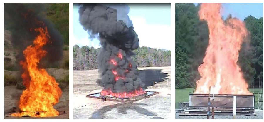
Dutch Diesel ~6 ft diameter (1.8 m) Dahlgren JP5 12ft x 12ft (3.8 x 3.8 m)
