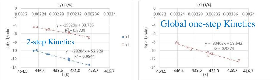
Thermal degradation rate increases with confinement
