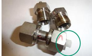
Vented Test Con115: 2.93% mass loss
