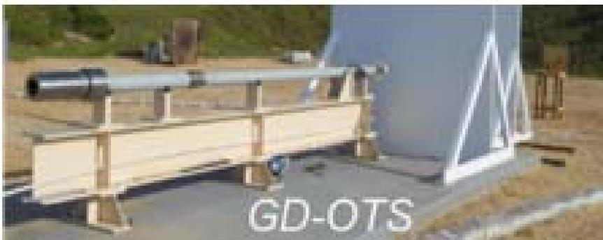
Figure 2. Typical fragment impact test setup
