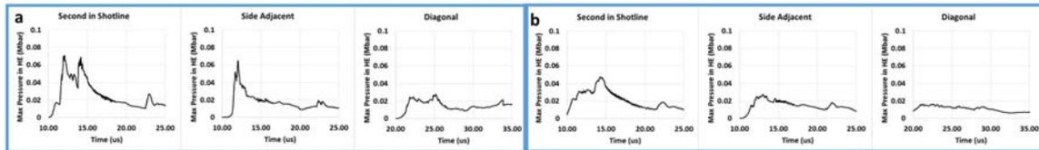
**Figure 12. Maximum pressure in HE region (Mbar) vs. time (us) plots for cartridges, (a) baseline and (b) plastic barrier configurations**
