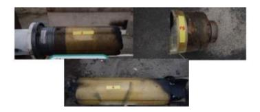
→ Classification : Type IV instead of Type V expected due to test bench attachment mean
