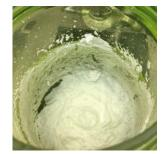
If lacquer was added to a warm (60 °C) slurry, the binder becomes associated with the water phase and coats the vessel rather than forming beads.
