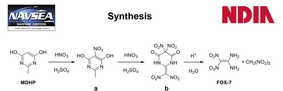
Mixed acid nitration conducted at 10-30°C
