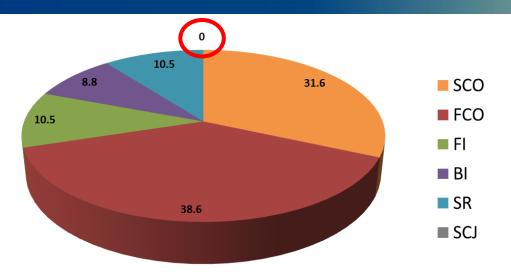
→ About 70 % of the existing mitigation technologies for SRMs are designed against thermal threats (FCO and/or SCO) although the impact threats (BI, FI, SR and SCJ) are considered as a critical issue for rocket motors, especially in the case of minimum smoke ones:
