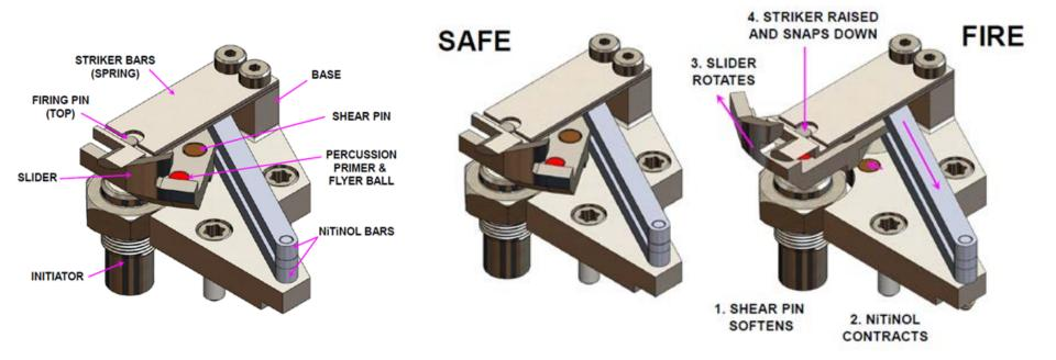
Sain, J., Sanford, M., Active Mitigation: Rocket Initiator Thermally Activated (RITA) Insensitive Munitions (IM) Device for the MK22 Mod 4 Rocket Motor, FUZE 2012
