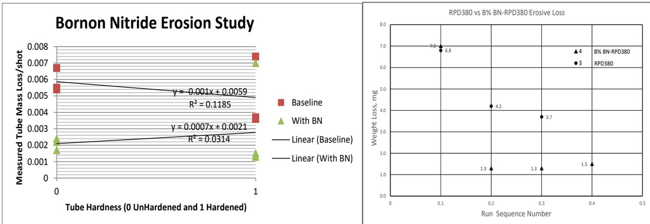
**Figure 12:** Wear and Erosion Test Results for hard and unhardened sleeves (US Patent Pending). Note: Sleeves 1 and 2 were hardened to approximately Rockwell Hc 41. Sleeves 3 and 4 were approximately Rockwell Hc 12.
