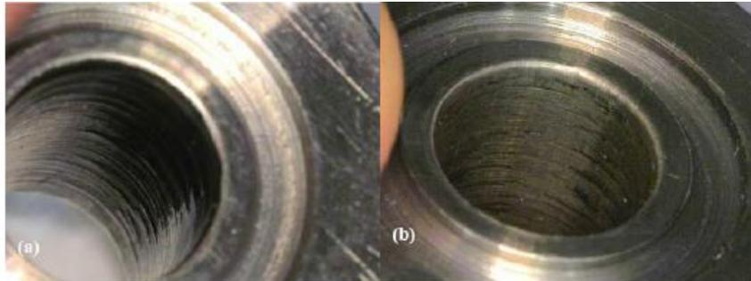
**Figure 5:** Insert Sleeve 2 – (a) hardened Steel, after firing 3 shots RPD380 Propellant (Cleaned) RPD380 P - Flow Entrance End –cleaned after 3 shots (b) RPD380 P - Flow Exit End –cleaned after 3 shots
