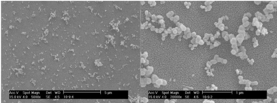
**Figure 6:** Scanning electron micrographs of BN nano-particles (US Patent Pending) used for propellant additive testing.
