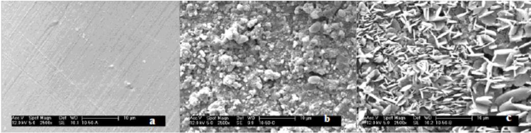
**Figure 11:** SEM images of (a) unfired steel insert (b) steel insert fired with 5 grams of IMR-4198, and (c) steel insert fired with 5 grams of B% BN composite propellant.
