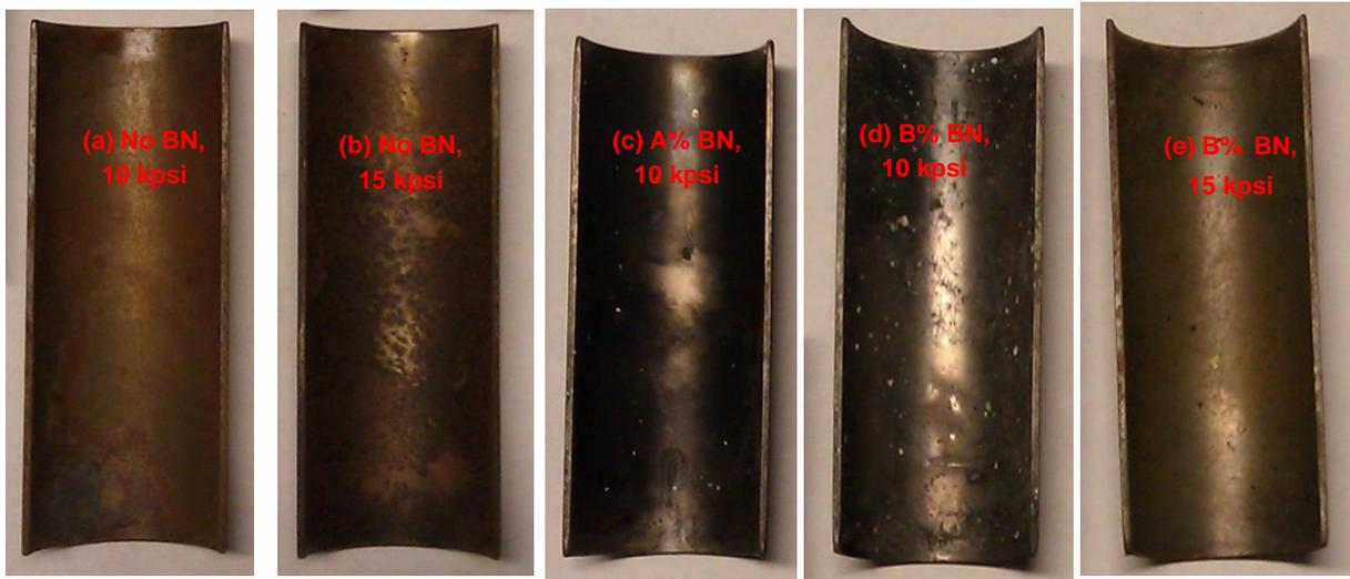
**Figure 9:** Photographs of steel inserts after closed bomb testing at ~10,000 psi and ~15,000 psi; listed in Table 1; Steel inserts after bomb testing samples fired with a composite propellant containing BN (A<B) had less oxidation than sample fired with pure propellant.
