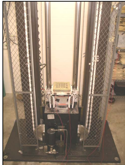
High-g Shock Tower (simulate gun-fire conditions)
