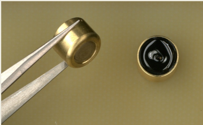
Finish and tested laser diode primer
