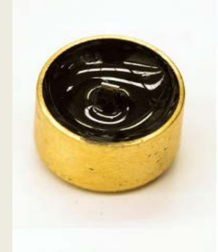
Assembly mounting, post potting
