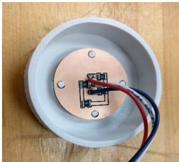
Printed mold; Traditional PCB (FR-4)
