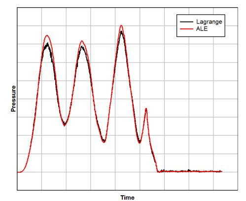
Pressure Exerted on Embedded Brick versus Time
