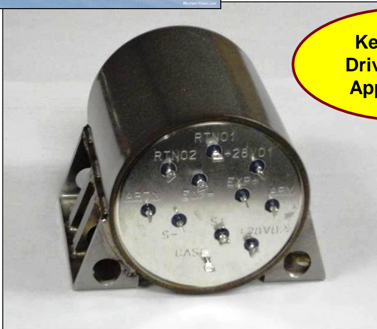
LiSi/FeS 2 FTS Thermal Battery (Device No. G3206A1)
