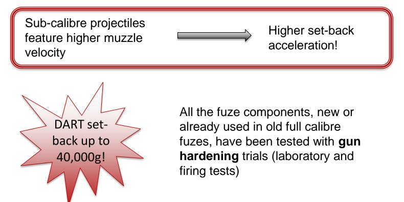
NOTE: in-barrel lateral accelerations are also greater than for full calibre!
