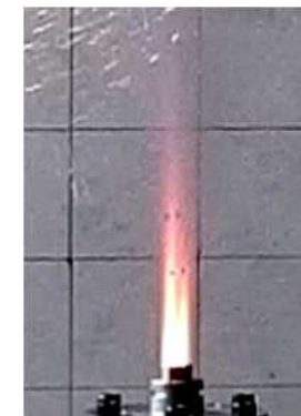
Firing of LEEFI igniter (for propellant)
