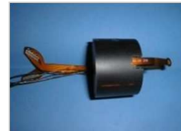
FBM21 Electronic Module including Fireset
