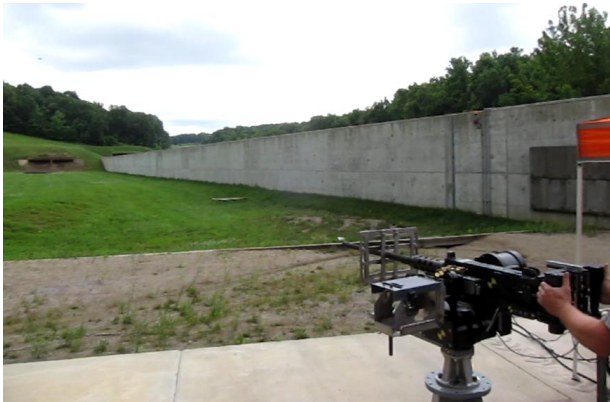
Live-Fire testing of .50 Caliber M2HB Machine Gun on Flex Force Maritime ASP
