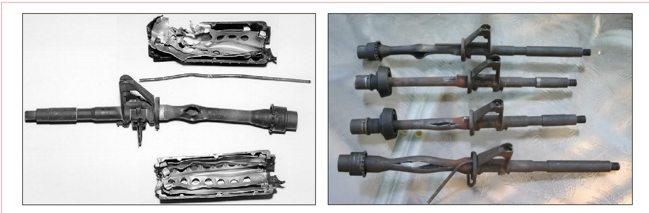
Above: DoD M-4 Barrel Failure With Forend; AR-15.com Four Failed M-4 Barrels In Reduced Diameter Section.
