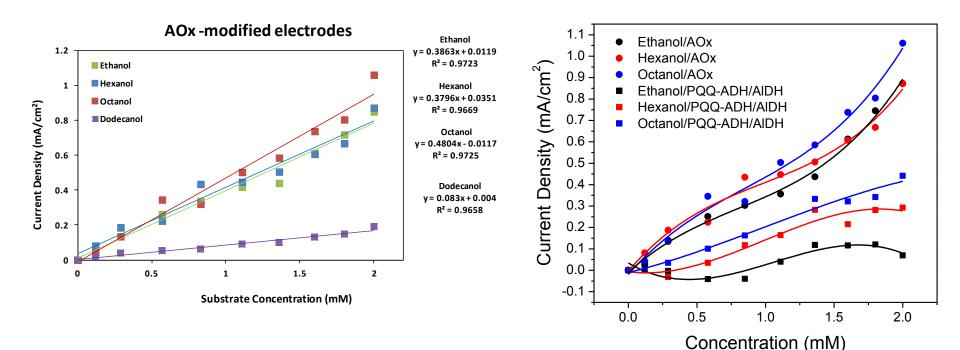
AOx converts C2, C6, C8, and C12 alcohols to energy. Lower eff. for C12 process. AOx – single step oxidation of alcohol to aldehyde.
