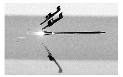
An image of sabot separation from a high velocity long rod penetrator [1].
