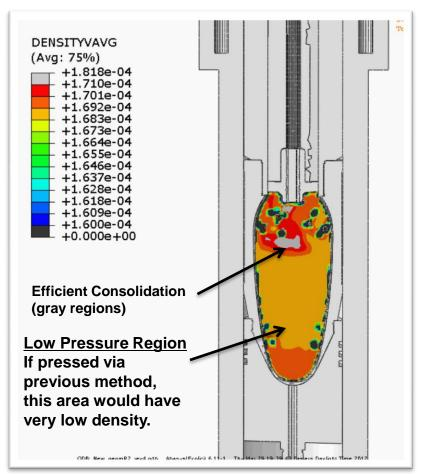
• Efficient consolidation may only be achieved if the punch diameter is equal to or greater than the length of container (length/diameter L/D less than 1).
