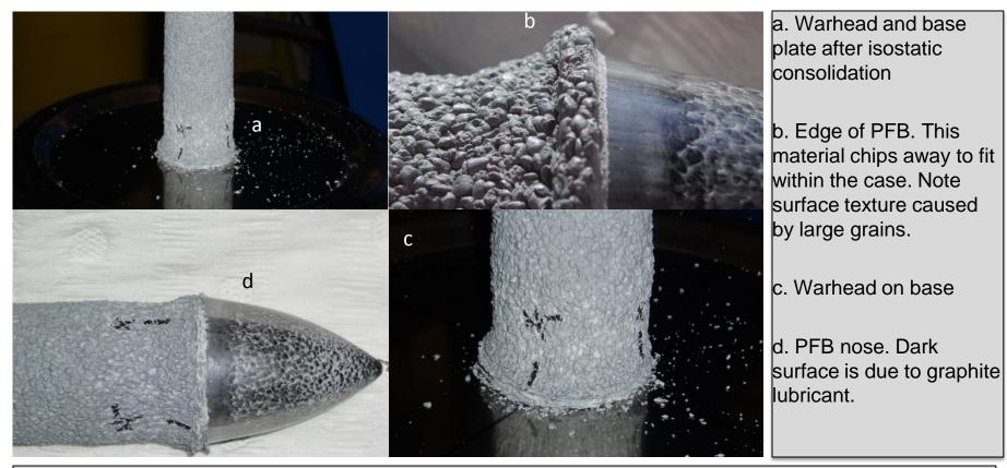
The explosive used in development of this process was PAX-3, an Aluminized HMX composition. It is known empirically to flow well, but further study is needed to determine exactly what mechanical properties respond best to the single-increment process.
