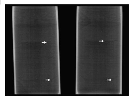
The pressed Warhead shown here was pressed incrementally. Density gradients and cracks have formed at the boundary of each increment.
