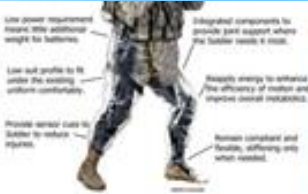
The CASPA Warrior Web concept aims to develop a skin suit with embedded technology to reduce Soldier injuries while maintaining Soldier performance.
