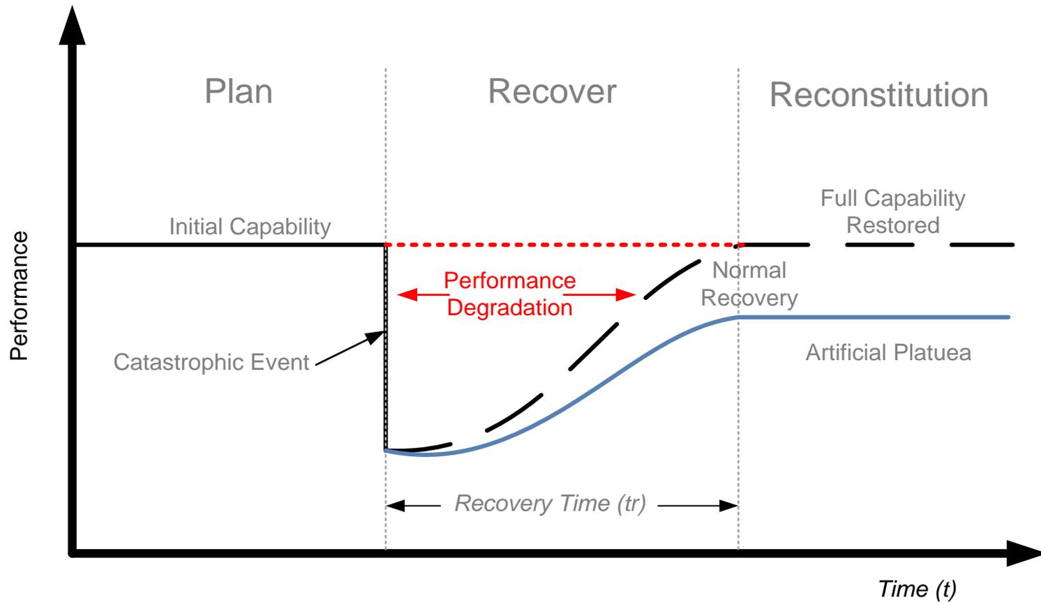
**Artificial Plateau - System does not recover to original performance level.**
