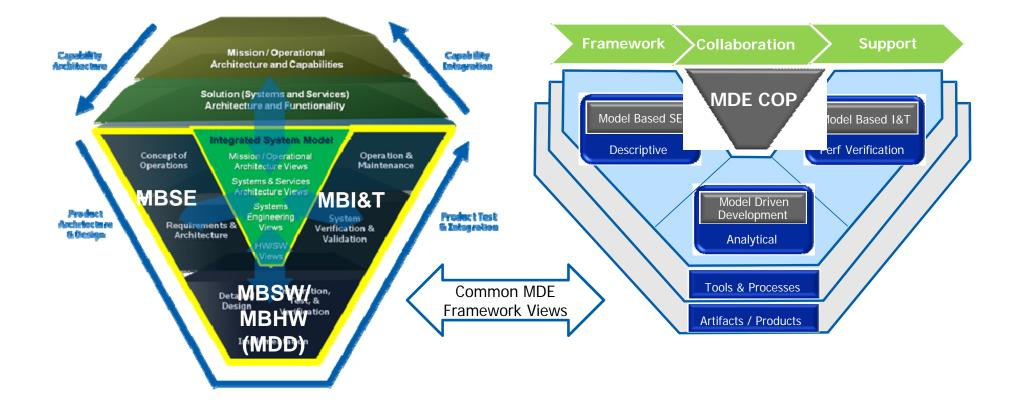
MDE includes Model-Based Systems Engineering, Model Driven Development, and Model Based Integration and Test
