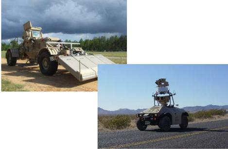
**Force Protection:** Threat Detection and Neutralization for Route Clearance efforts demonstrate and matures threat/mine detection and neutralization capabilities to address a broader spectrum of in-road threats for route clearance vehicles. Base protection capabilities such as MDARS (Mobile Detection Assessment Response System robot) are useful for patrolling remote areas.
