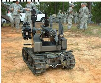
**Force Application:** MAARS (Modular Advanced Armed Robotic System) is the first fully modular ground robot system capable of providing a measured response including non-lethal, less-lethal and even lethal stand-off capabilities.
