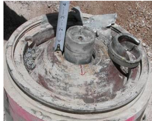
Fuze Expelled from Fuzewell in High G Characterization Tests
