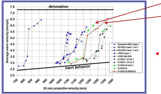
Shock sensitivity of VI-RDX produced at pilot scale quite similar to that obtained with the first ISL trial at 5 L. scale
