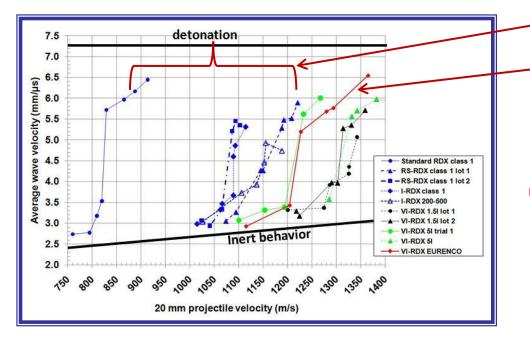
Shock sensitivity of VI-RDX produced at pilot scale better than that for commercially available RS-RDX or I-RDX<sup>®</sup>
