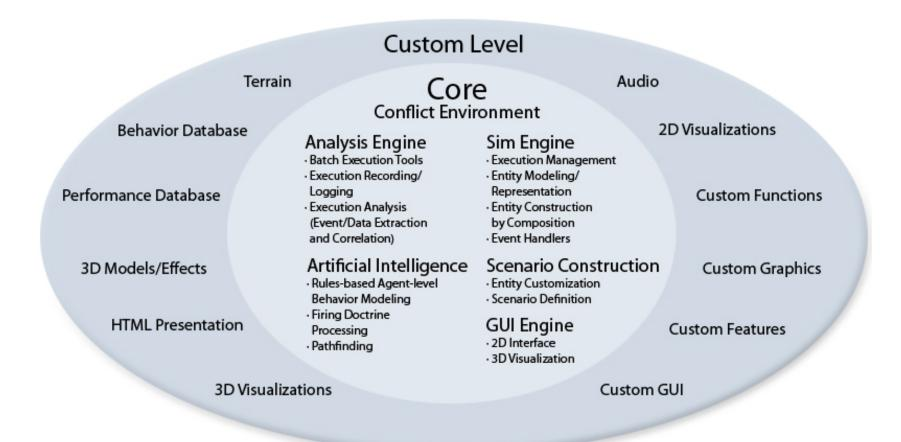
Core framework extended and customized by adding features via plugin architecture
