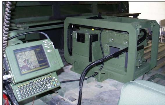
M111 Improved Position and Azimuth Determining System (IPADS)
