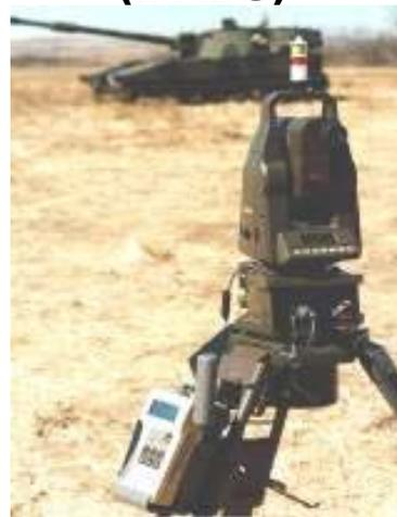
Gun Laying and Positioning System (GLPS)
