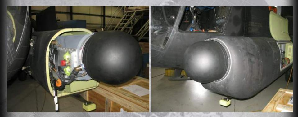
AN/APQ-187 Radar Installation On MH-47G
