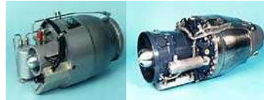
Low Cost Expendable Engines for Missiles and UAV's
