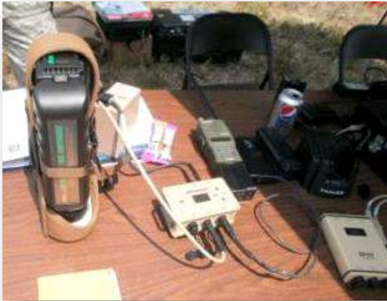
LWSB connected to AN/PRC-152, Protonix Power management unit and Ultracell Fuel Cell
