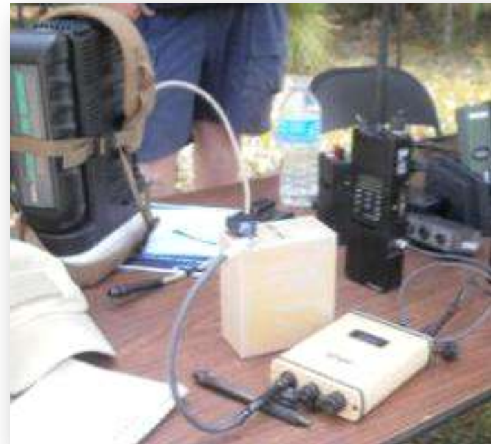
LWSB connected to AN/PRC-148, SFC Power management unit and XX-2590 battery
