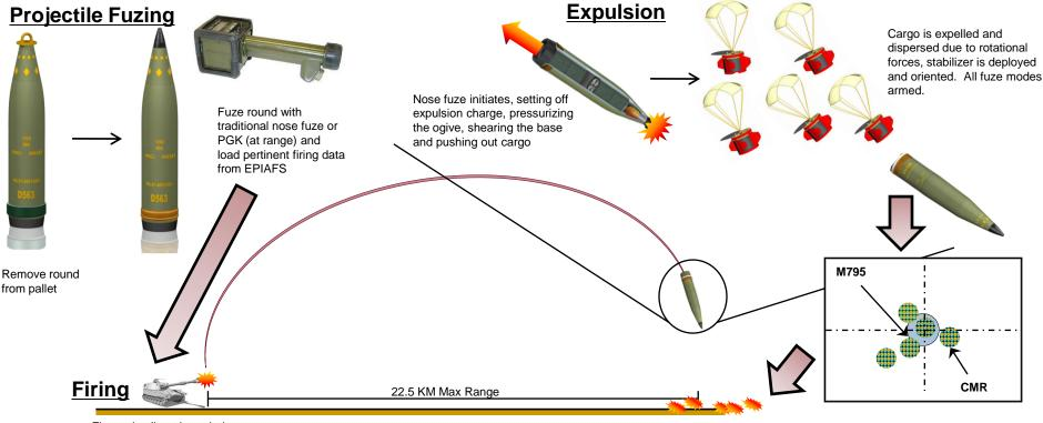
Fire projectile at intended target Fully zoneable up to MACS5
