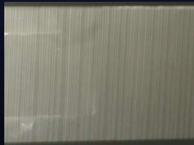
Matrix cracking in carbon fiber composite
