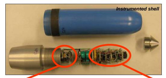
Instrumented functions (Impact detection + setback generator)
