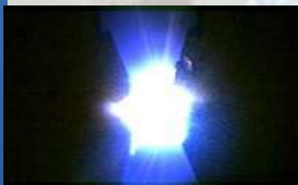
Vaporization of an IHDI MEMS initiator
