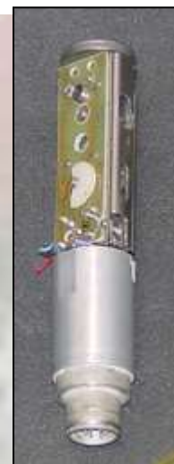
Complex Electro- Mechanical Safe-Arm Devices
