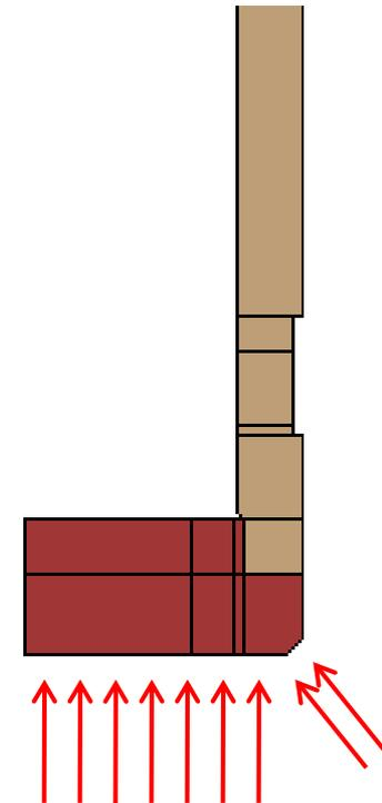
**Figure 4. a)** A surface force, simulating the Zone 7 propellant charge, is applied to the outer surface of the base of the projectile. The 105mm projectile experiences a maximum pressure of approximately 32000 psi for 6 ms. **b)** Zoom in of projectile base. Arrows depict force placement.
