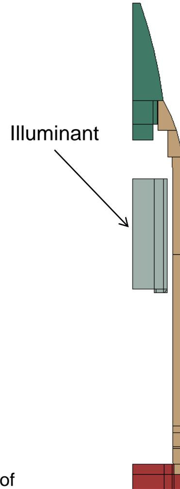
**Figure 1.** Fuze, projectile body, base and illuminant (gray) of 105mm projectile in half symmetry, axisymmetric model. The voids are locations for other ancillary components(not depicted).
