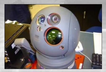
Ruggedized, Marinized, Light Weight, Gyro Stabilized, Cryogenically Cooled, Color & Infrared Camera, Laser Range Finder & Pointer
