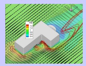
Developed for Exterior Stationary Grids 1.5M Cells 30 Seconds of Simulation Single CPU – 20K slower 7 Days of Runtime
