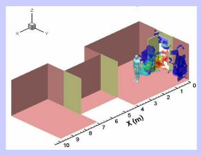
Developed for Interior Moving Man in Simulation 8M cells 10 Seconds of Simulation 50 CPUs – 4K slower 12 Hours of Runtime
