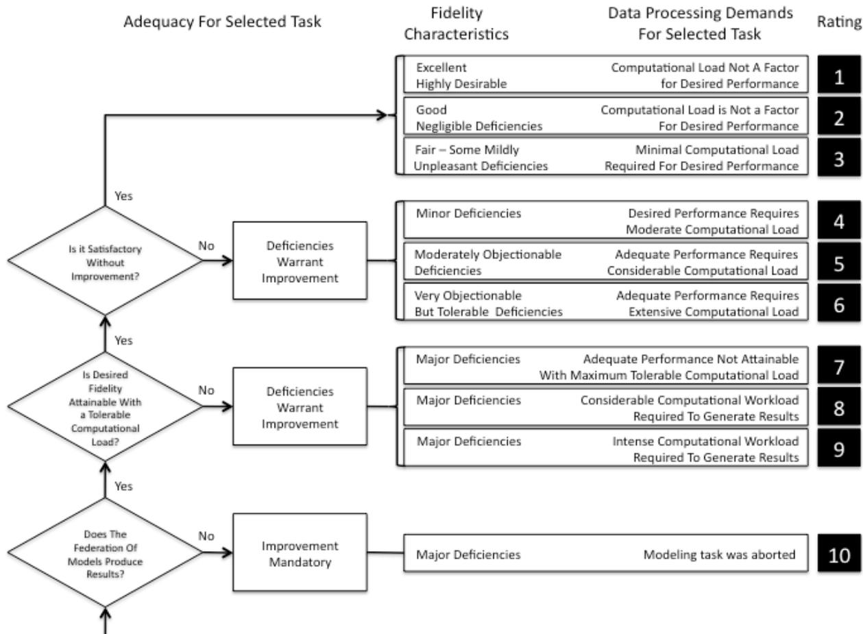
**Based on the Cooper-Harper Handling Qualities Rating Scale**
