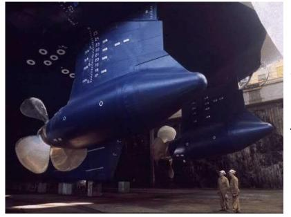
Ship electrically driven propulsion pod, rotates 360°, no rudder, eliminates need for tugs
